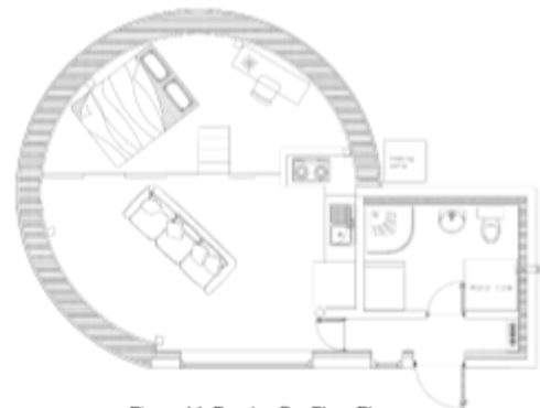
Figure 14: Passive Ger Floor Plan
